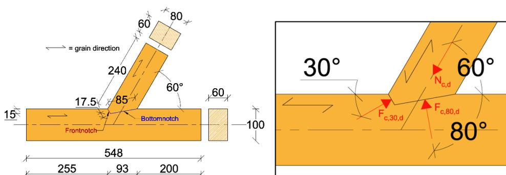
**Figure 1: Single notch joint**
