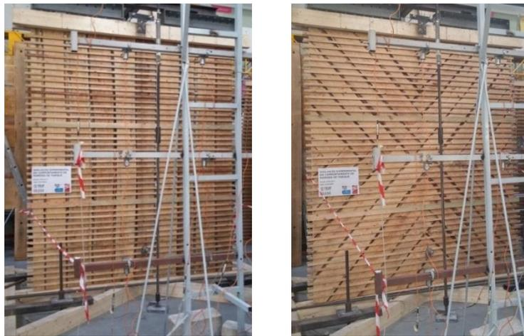
Figure 1 – TWs specimens
