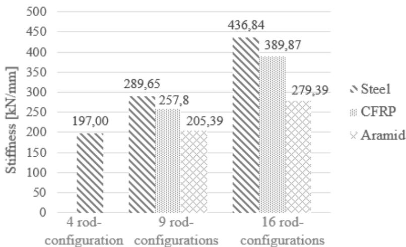
Figure 1 : Stiffness  $K_n$  connection of multiple glued-in rod connections [kN/mm]
