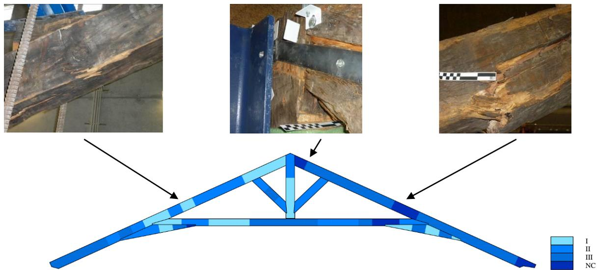
**Fig. 1** - Visual grading of truss T2 with details of the failure of the rafters and of the post-rafter connection.
