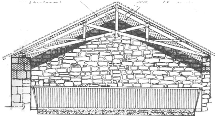
Fig. 2 – A 14.60m span scissor’s timber truss for the horse-riding building.
