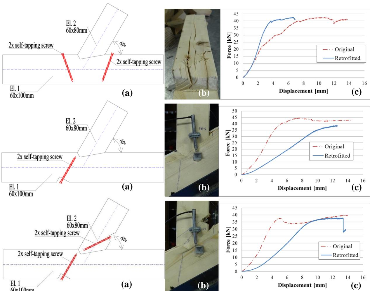
Figure 3: Retrofitting techniques 1-3 (a) retrofitting with self-tapping screws, (b) obtained failure and (c) comparison of force displacement relationship from loading cell for both original and retrofitted joint.
