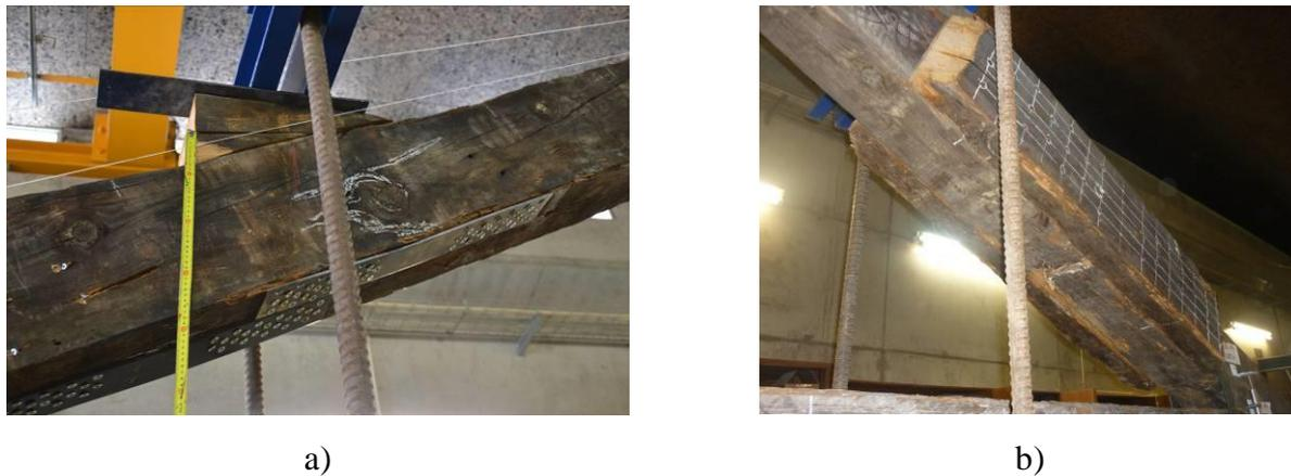
**Fig. 2** – Strengthening techniques with screwed: a) metal plates b) timber elements.
