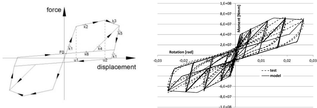
Figure 1: On the left: Florence pinching hysteresis model with six inclinations K1 to K6. On the right: Overlap of cyclic tests on Borbone wall and numerical model.
