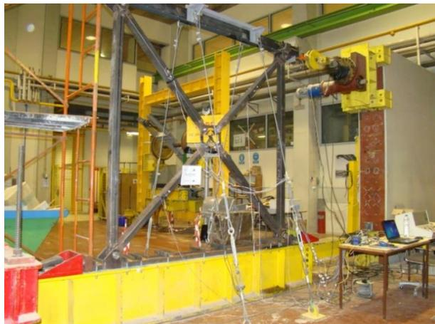
Figure 2 – Experimental setup for testing the Dissipation Panels.
