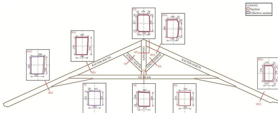
**Fig. 1 - The collar truss with representative sections obtained from the geometrical survey mapped.**
