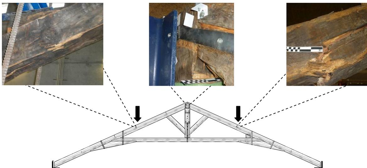
**Fig. 1** - Schematic of test setup and details of the failure of the rafters and of the post-rafter connection
