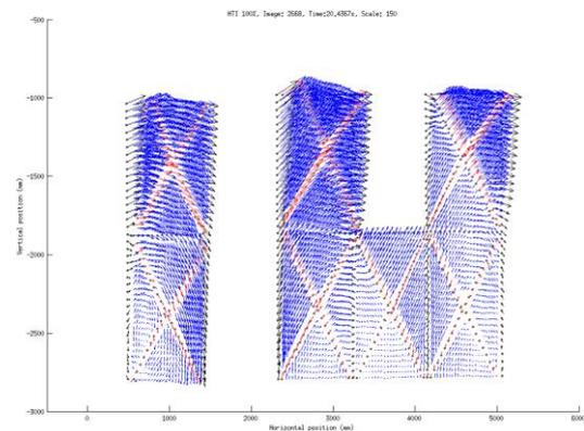
Fig. 3. Vector displacement with DIC measurement
