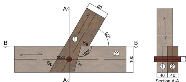
**Figure 1: Geometry of tested dovetail joints with the dowel**
