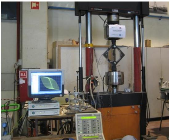
Figure 1 – Experimental setup for testing the Hysteretic Dampers.
