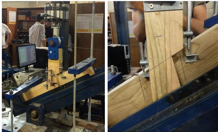
**Figure 2: Dovetail joints with and without dowel during experiments**
