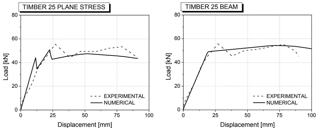
Fig. 1 Model calibration: plane stress elements (left) and beam elements (right) model results
