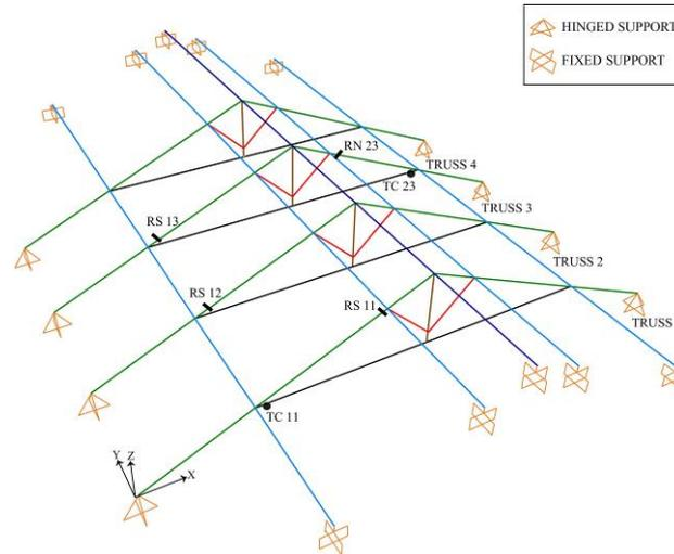
**Fig. 2** – Finite Element Model of the roof structure
