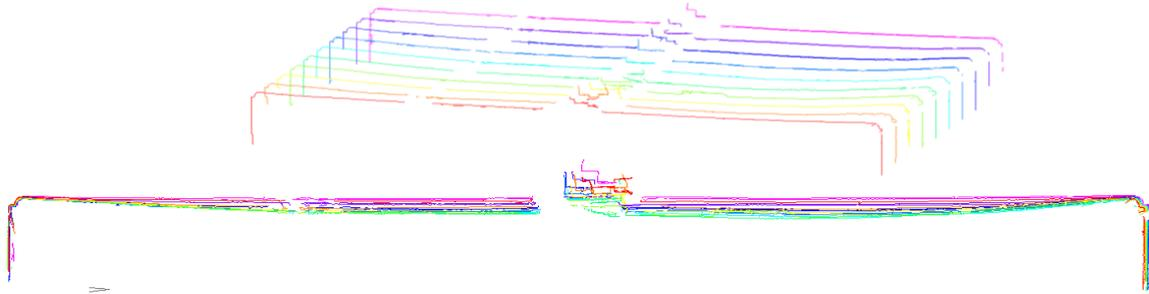
Fig. Progression of cross section through ceiling and wooden structure, in a 3D spatial view (top) and a planar view (down) in which it is visible the depression of the wattle dropped ceiling surface.
