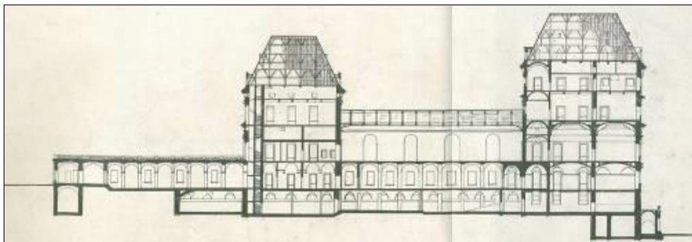
Fig. Timber roof structure of the Valentino Castle in Turin
