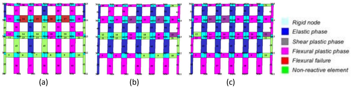
Figure 3 Damage pattern for front façade for triangular load in X direction: (a)Original; (b)  $R_{max}$ ; (c)  $R_{min}$
