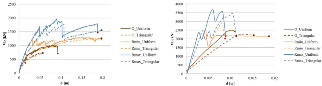
Fig. 2 Pushover curves: X (left) and Y (right)direction
