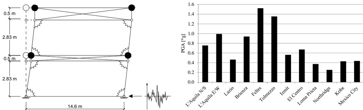
Figure 2: 2D model of case study building (on the left) and maximum sustainable PGA values of Borbone case study (on the right).
